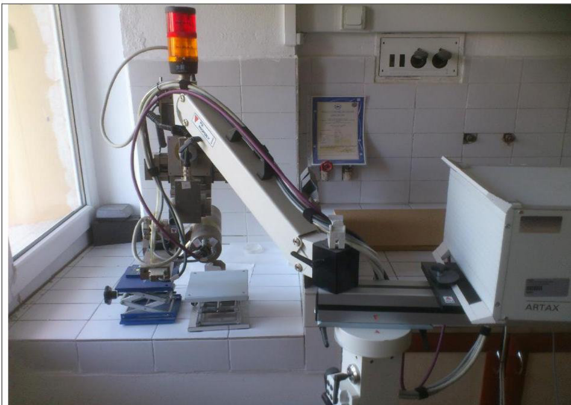
Figure 2 Artax 800 \mu -XRF Instrument for rapid point analyses and elemental mappings
